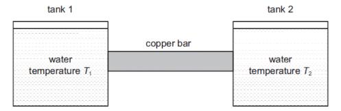
The temperature of the water in tank 1 is  $T_1$ . The water in tank 2 is at a higher temperature  $T_2$ .
