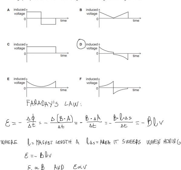
The induced voltage is proportional to B and v.
