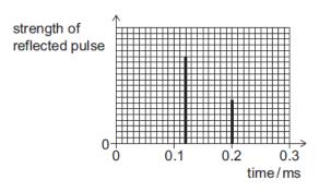
The speed of ultrasound in the metal is 5000 m s<sup>-1</sup>.
