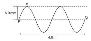
At time t = 0 ms, point X on the string is at its maximum displacement of 6.0 mm above equilibrium.
