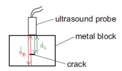
On the way to the crack, the ultrasound wave travels there and back, therefore a distance of  $2d_C$ . It is received first, at  $t_1$ =0.12 ms, because the crack is closer to the probe.
